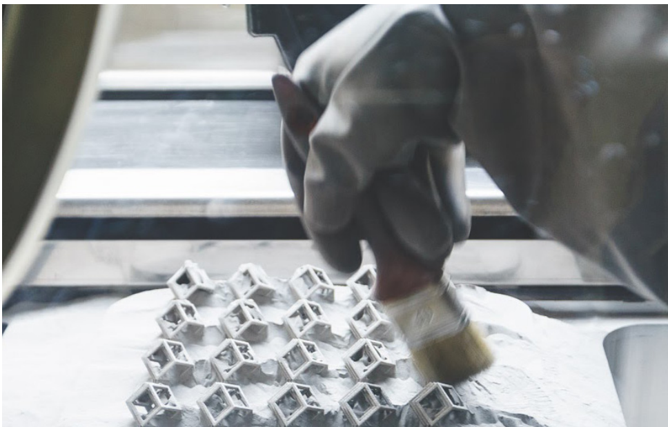
Powder removal after printing. Build plate contains 20 custom parts in steel.
