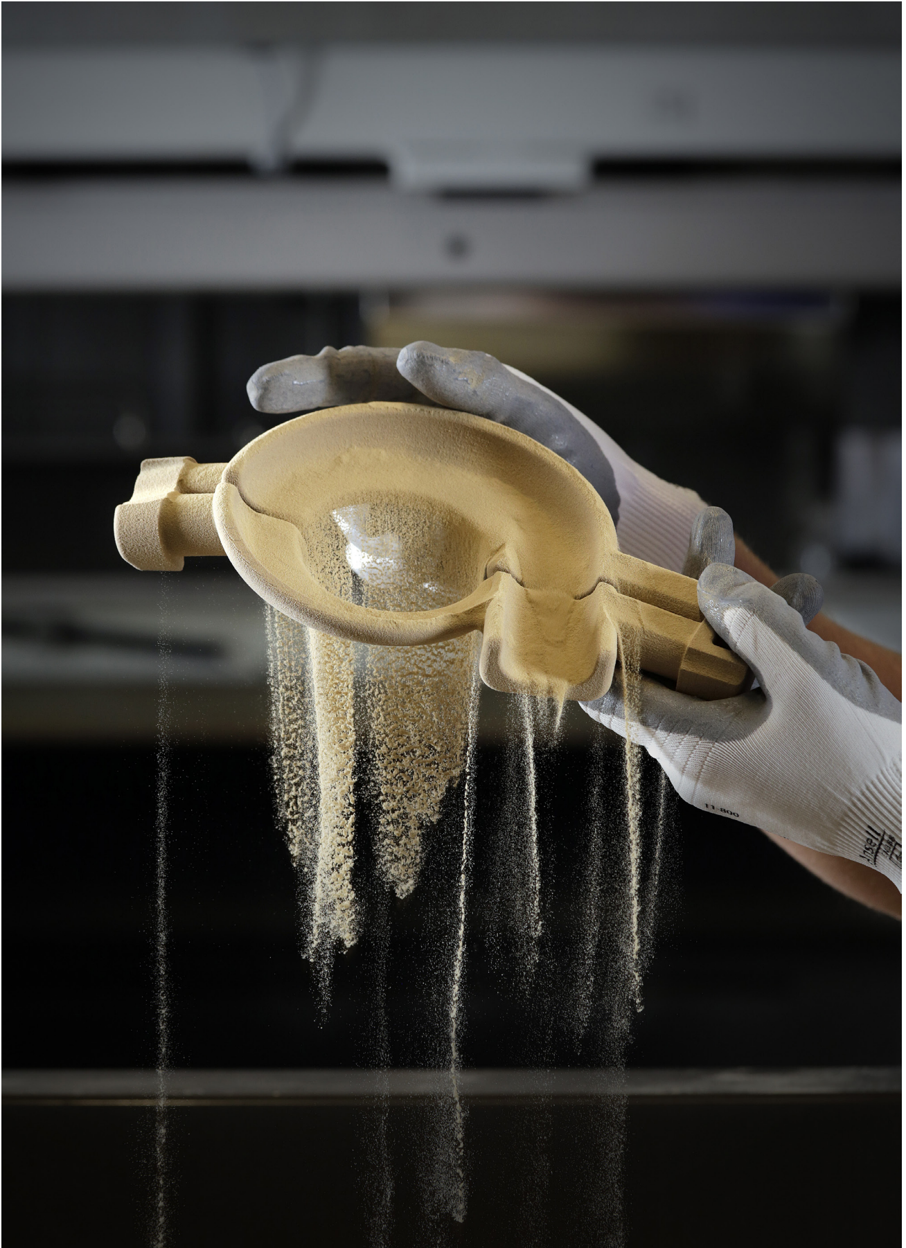
Binder Jetting part taken out of the powder. Image courtesy of ExOne.
