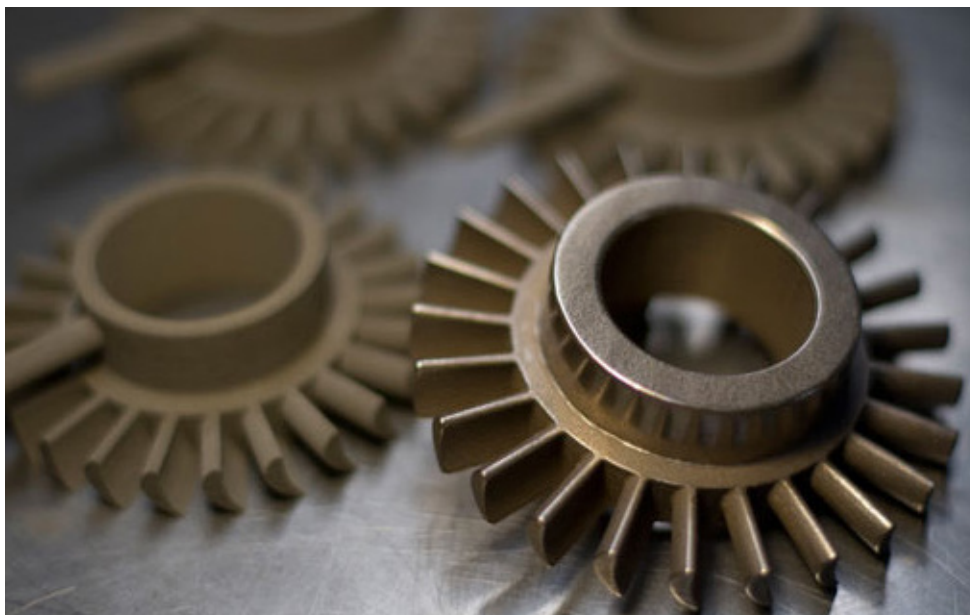
*Binder Jetted metal parts. Before secondary processes (left) and after infiltration and tumbling (right). Image courtesy of ExOne.
