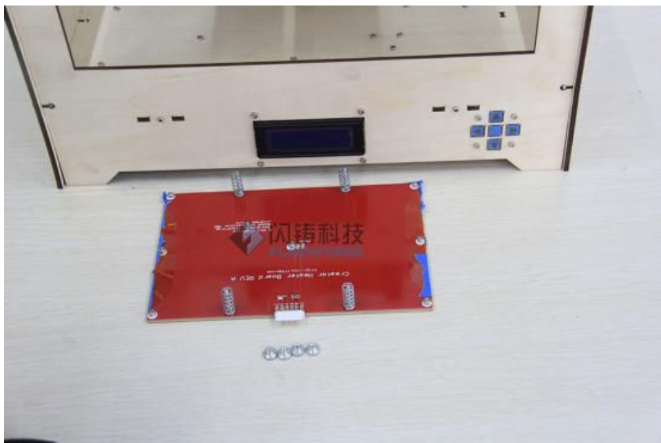
Replace the new heating plate
