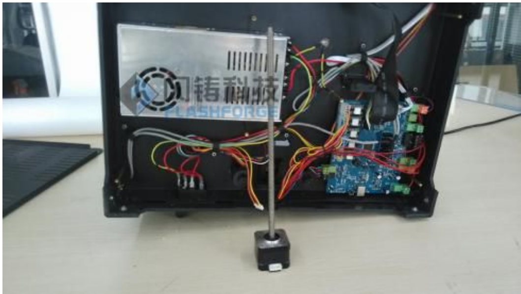
Replace with a new motor
