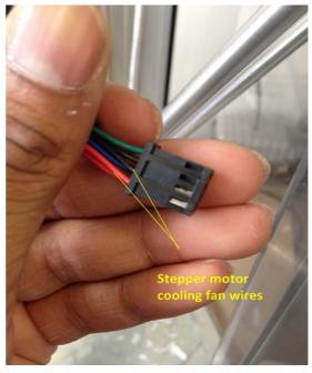
4. Now, check the connections on your extruder connector as they should match the combination shown in the above pictures. If any of the wire is not in combination then you need to disconnect that individual wire and swap it accordingly, further if the wires are in combination as shown but
