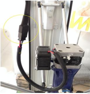
2. Use a safety knife or a blade to carefully cut and remove the heat shrink tube as shown in the picture. Make sure to cut the heat shrink very gently to avoid cutting the cable wires.
