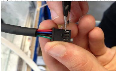
6. Insert the Pink wire of the extruder cable into the connector from which you removed the Black one. To do so, very gently bend the metal tab on the crimp outwards using your finger nail, and carefully slide it into its connector. You should hear a soft 'click'.
