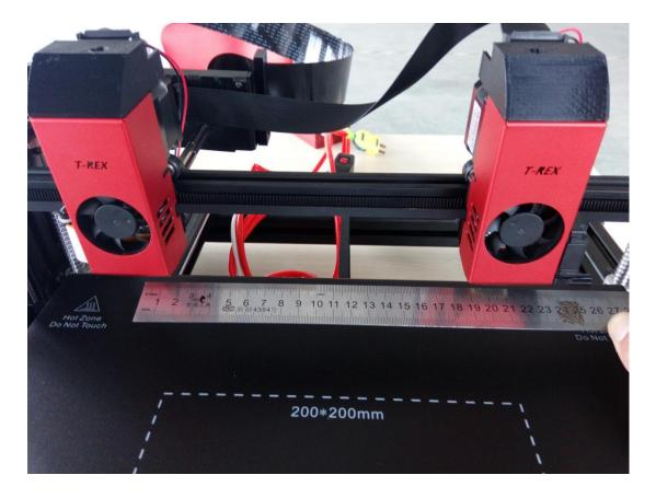
Then connect the flat wire of right extruder to E0a or E0b.
