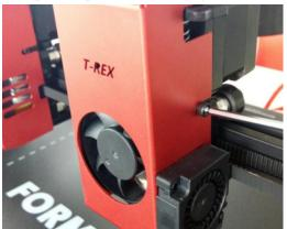
Then tighten below two screws to fix right extruder on synchronous belt.
