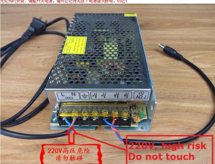
按下图所示,把电源线、DC线按指定颜色接入开关电源对应位置的接线端子,请勿将电线金属部分暴露在外! 无论何时安装、调整开关电源,请务必记得先拔下电源插头断电,切记! 3, Third step,Connect white plus hotline to HOT BED terminals, red and black temperature cable into TB horns socket.
