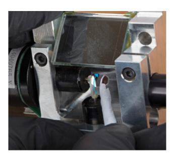
If it is necessary to clean the mirror, carefully position the galvo block as shown. Use the swab to gently rotate the mirror so that the surface is more easily accessible. Gently wipe the mirror from the base of the mirror to the end of the mirror. Rotate the swab and wipe again.
