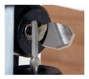
Once the mirrors are clean, the galvo block can be reinstalled into the Form 1+. Use a bright light or flashlight to illuminate the mirrors.
