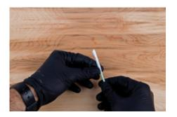
Secure the PEC-PAD strip at the bottom of the shaft with another piece of small tape. When finished, it should look similar to the one shown.
