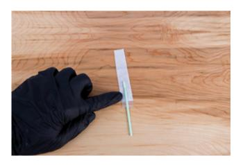
Cut a strip about 1cm wide out of PEC-PAD. Lay the swab stick on the PEC-PAD as shown above. Apply a piece of tape extending beyond the length of the PEC-PAD strip.
