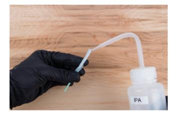
Apply a small amount of isopropyl alcohol to the PEC-PAD swab.
