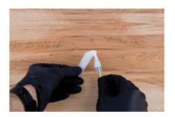
Fold the end of the PEC-PAD over to the side. Begin wrapping the PEC-PAD tightly down and around the shaft as shown.
