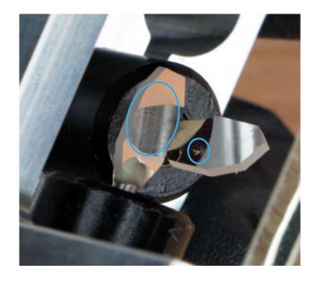
Closely inspect the mirrors for any signs of particles, dust or residue. Use a bright light or a flashlight to illuminate the mirrors.
